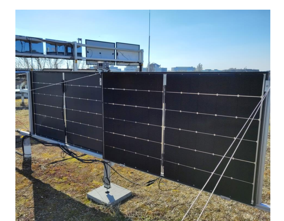
Fig. 5 (above): Picture of the SHJ bifacial PV modules (now mounted facing east/west)
