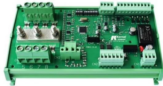
Figure 6: Kernel ST2 0825 string monitoring device
