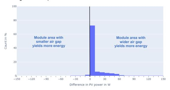
Figure 32: Difference in PV power from two different facade substructure variations (02.01. - 02.04.2022)
