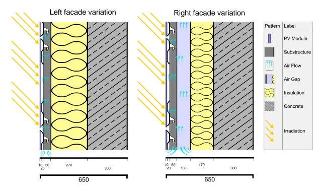
Figure 4: Schematic facade cross section of both variations of the module substructure
