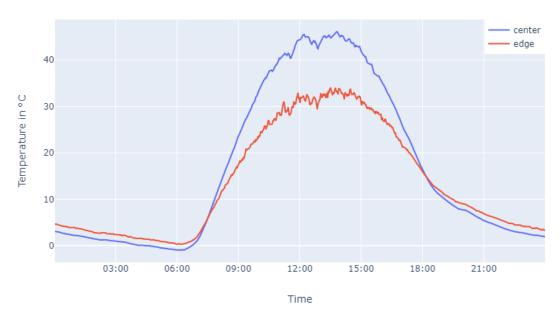
Figure 34: Single defective sensor for the edge module temperature measured at a selected PV module at the bottom on the  $24^{\rm th}$  of March
