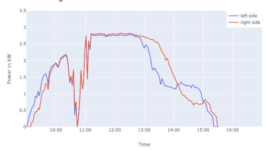
Figure 30: PV power from two different facade substructure variations on the 25th of December
