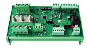
Figure 6: Kernel ST2 0825 string monitoring device
