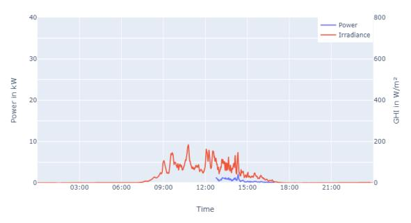
Figure 13: Total PV power in the area under investigation in contrast to the irradiance on the 16th of February
