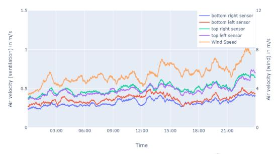
Figure 24: Average air velocity of the rear-ventilation and the ambient wind on the 16th of February
