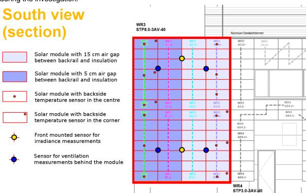
Figure 10: Sensor placement in the area under investigation
