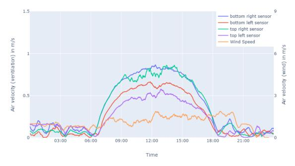
Figure 23: Average air velocity of the rear-ventilation and the ambient wind on the 24th of March
