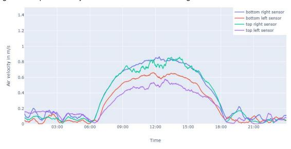
Figure 20: Average air velocity of the rear-ventilation on the 24th of March
