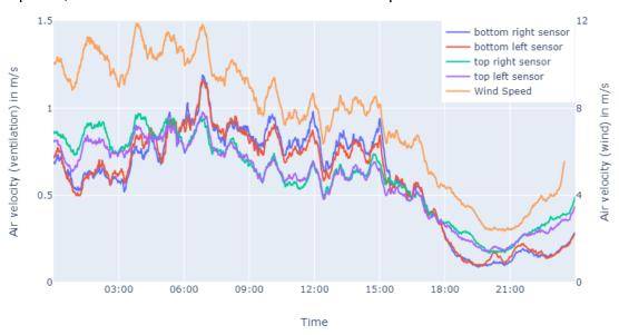
Figure 25: Average air velocity of the rear-ventilation and the ambient wind on the 16th of February
