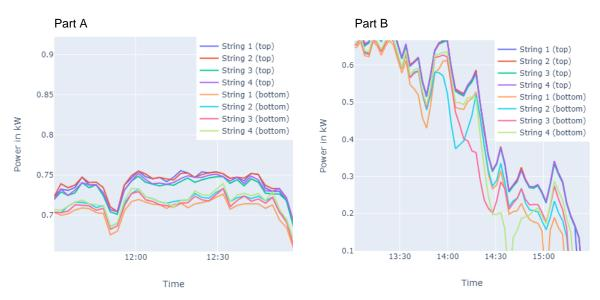
Figure 14: PV power in the area under investigation for each string on the 13th of February
