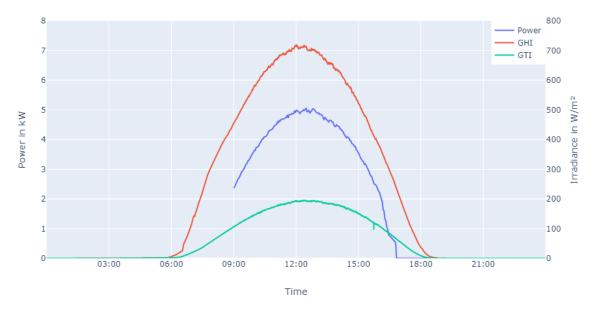
Figure 12: Total PV power in the area under investigation in contrast to the irradiance on the 24th of March
