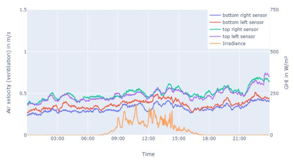
Figure 22: Average air velocity of the rear-ventilation and global horizontal irradiance on the 16th of February
