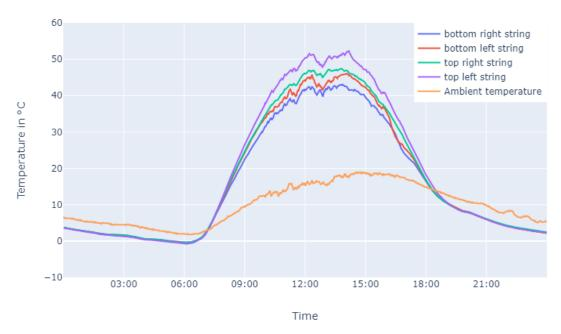
Figure 28: Average string temperature in contrast to the ambient temperature on the 24th of March
